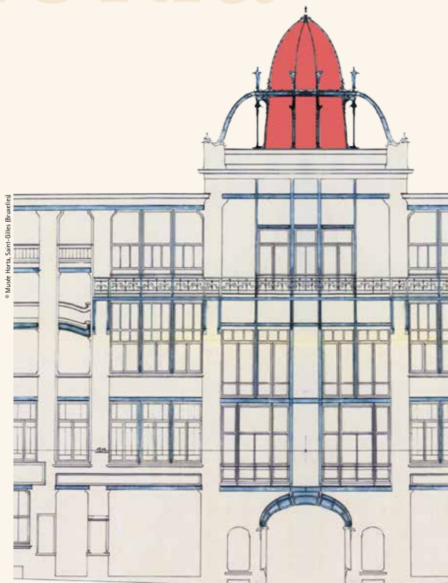
A digital simulation of a project drawing from 26 March 1896 recreates the dome's glazed red brick
