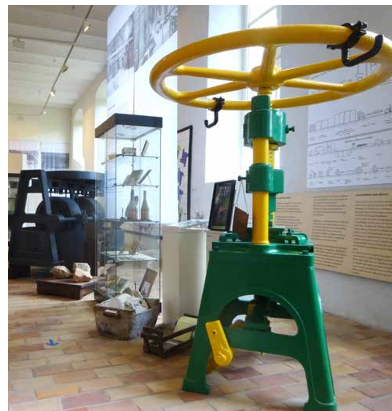
Manual tile press manufactured by the English company William Boulton Ltd, now on show at the Gilliot & Roelants Tile Museum
